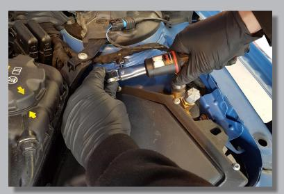
**Overview:** A fairly recent addition to the New Professional family is the Model 25 torque wrench. With its automotive ratchet, comfortable handle design and proven mechanism, this new torque wrench can be trusted to deliver accurate results on threaded fasteners. It is really at home in engine bays performing work in restricted spaces tightening fasteners to a high level of accuracy.
